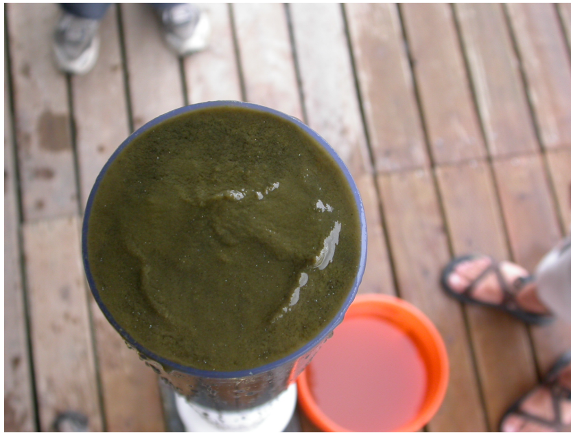
Figure 10. View of sediment core looking onto the surface of the sediment after draining the overlying water.
